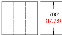
GI-700-750/257 DS .700" (17,78) LONG .750" (19,05) Ø O. D. .257" (6,53) Ø I. D. DELTRIN SPACER
